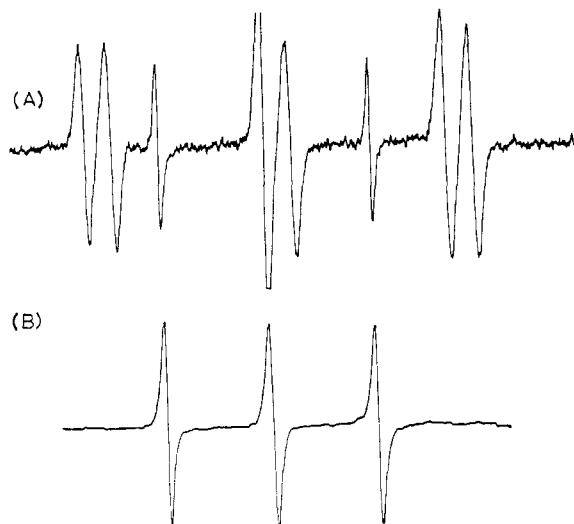
Figure 3. (A) The esr spectrum obtained from a solution of di- n -butyllead dichloride and phenyl- t -butyl nitron in benzene. (B) The esr spectrum of benzoyl- t -butyl nitroxide obtained from the addition of chlorine to phenyl- t -butyl nitron in benzene at room temperature.
